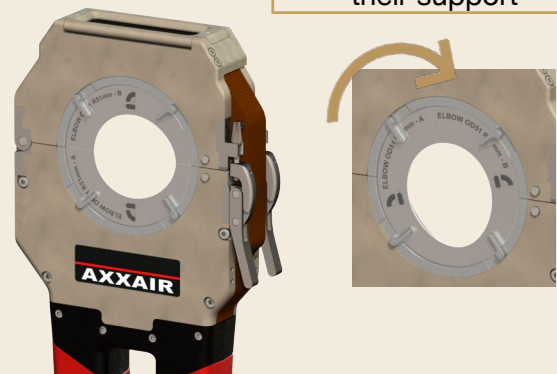
Elbow flange rotation on their support
