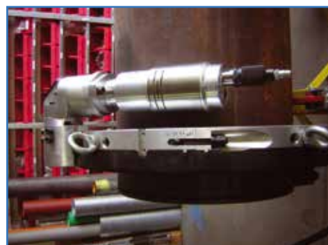
Angle gear for limited access on pipes and pipelines
