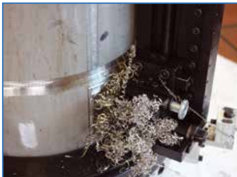
Removal of longitudinal weld seam
