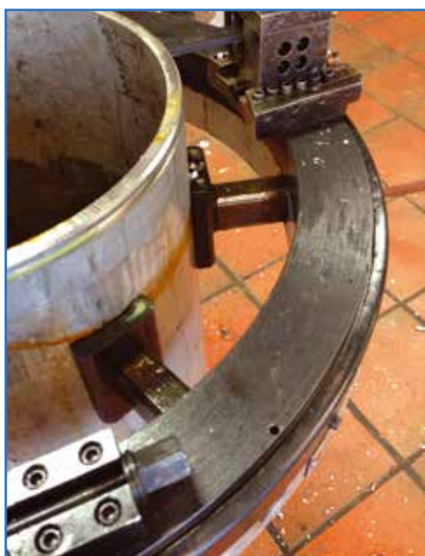
Special feet for thin wall pipes
