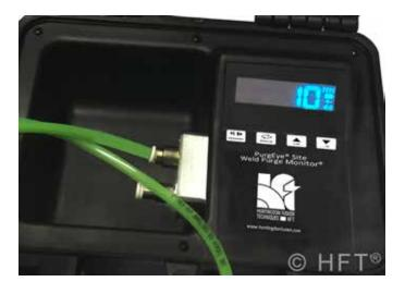
The **PurgEye® 1500 Site IP68** Weld Purge Monitor® can be used as a continuously reading instrument with free flow of the purge exhaust gas across the sensor, or as a sampling instrument with the integral electro-mechanical vacuum pump.
