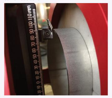
Tube with small diameters <25.4 mm are particularly concerned by the facing process. They are often cut with tube cutters or abrasive cutting machines. Generally speaking, tube must be faced before welding in order to obtain quality welds.
