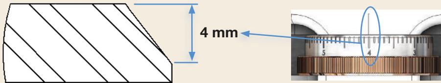
The vernier value is equal to the **bevel height**.
