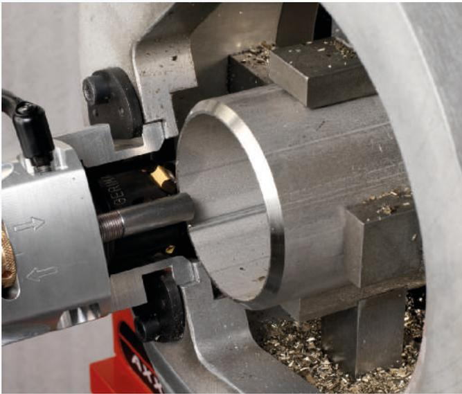
Above a thickness of 3 mm, simple fusion involves a melt volume that is too significant to guarantee proper geometric control of the weld bead. To remedy this, beveling reduces the quantity of material to be fused in order to achieve proper penetration.
