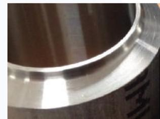
As the accessories (elbows, T unions, flanges, etc.) are generally prepared with V-bevels, many welds will need to be of the V-J type, which is difficult to achieve. Consequently, the quality of orbital welding accessories is generally a key criteria to be taken into consideration.
