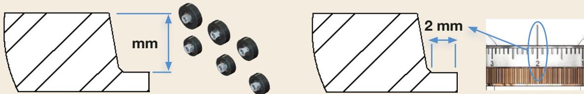
The value of the vernier is equal to the **length of the root face**.
