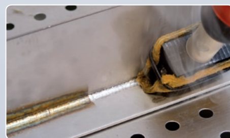
Old method: Welding seam cleaning with tampon
