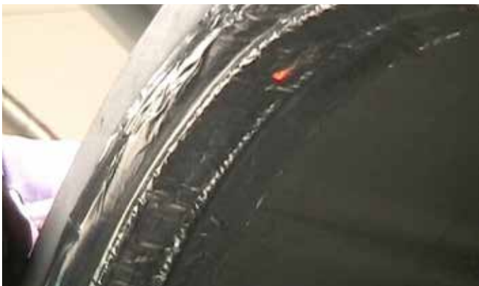
Step 2: Weld onto the Argweld® Purge Tape ®
