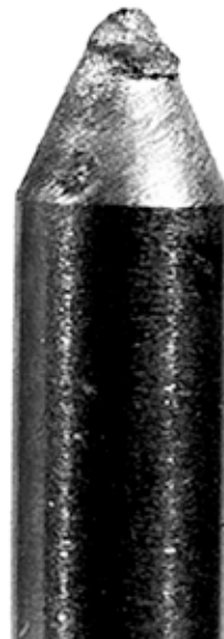
2% Thoriated Tungsten after 20 automatic welds
