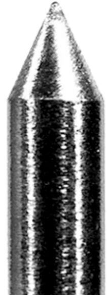
MultiStrike® Tungsten after 200+ welds
