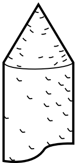
2% Thoriated Tungsten showing risk of uneven thoria distribution
